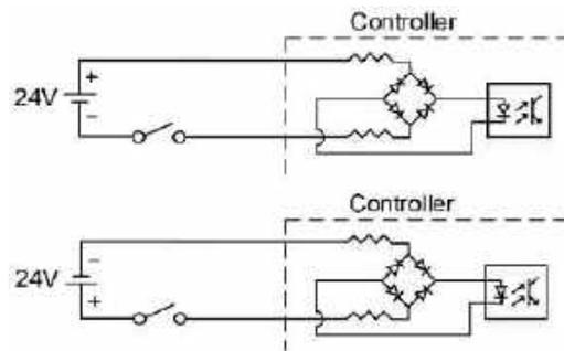
Note: the connection direction of the external power input for HSI does not affect the operation.
