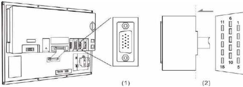
(1) Spindle analog output pins (female); (2) Spindle analog output pins (male)
