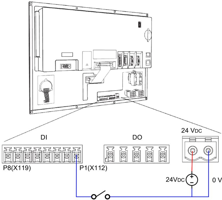
DO wiring (machine operation panel B supplies 24V power to the local I/O connector)
