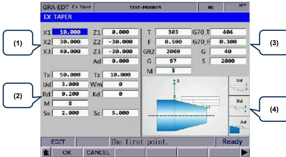
(1) Input fields for coordinates of each step point (You can leave the fields of items in blue blank, which means the points do not exist.)
