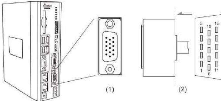
(1) Spindle analog output pins (female); (2) Spindle analog output pins (male)
