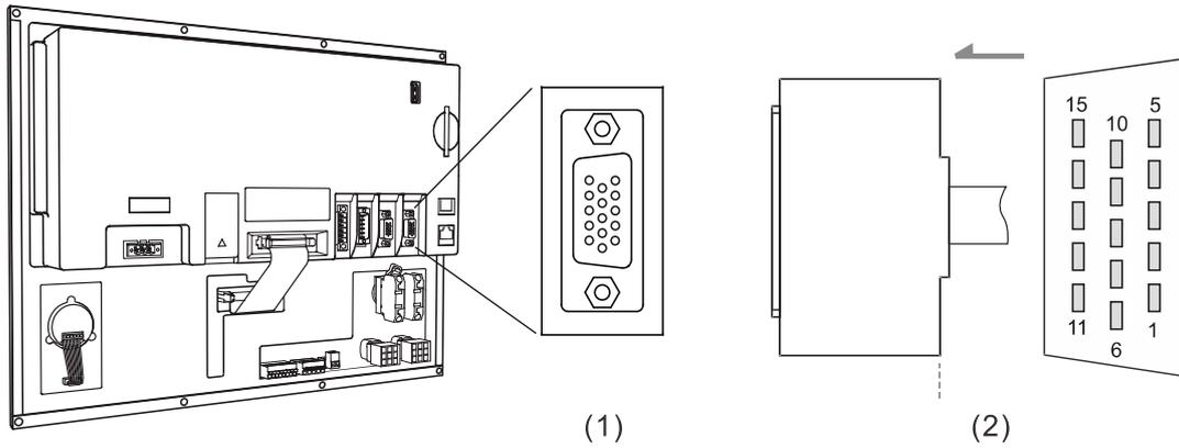
(1) MPG connector (female); (2) MPG connector (male)
