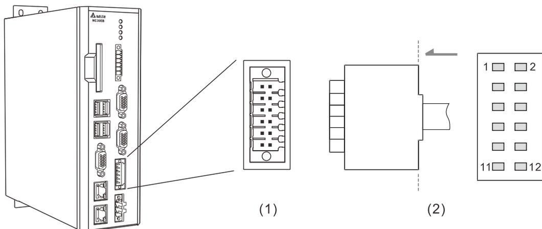
(1) CN1 connector (female); (2) Analog output pins
