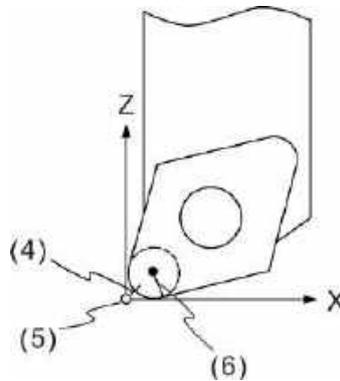
(4) Actual tool nose position; (5) Hypothetical tool nose position when calibration;
