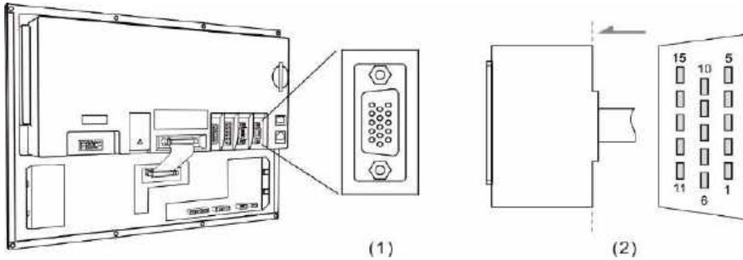
(1) MPG connector (female); (2) MPG connector (male)
