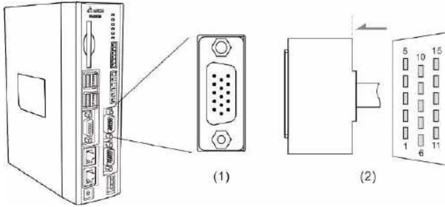
(1) MPG connector (female); (2) MPG connector (male)
