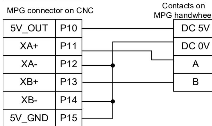
Wiring diagram for the pulse signals of the differential type MPG handwheel (EHDW-BE6SI):
