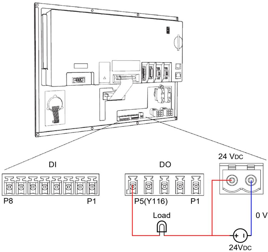
The pin assignment for the OPENCNC series models is as follows.
