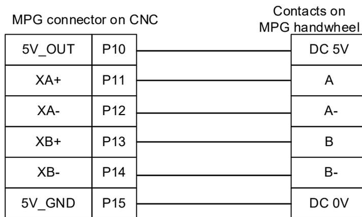
Wiring diagram for the MPG switch:
