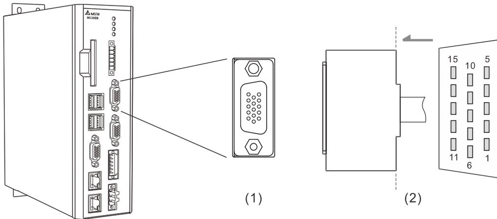
(1) MPG connector (female); (2) MPG connector (male)
