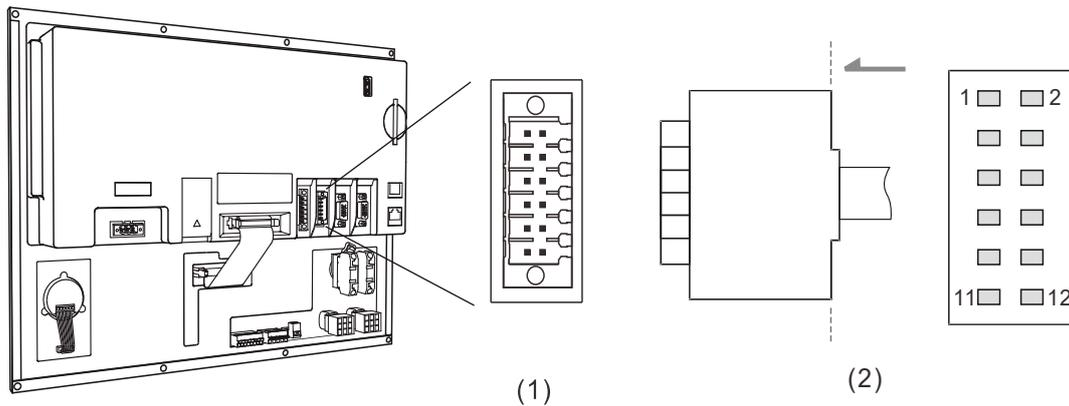
(1) CN1 connector (female); (2) Analog output pins
