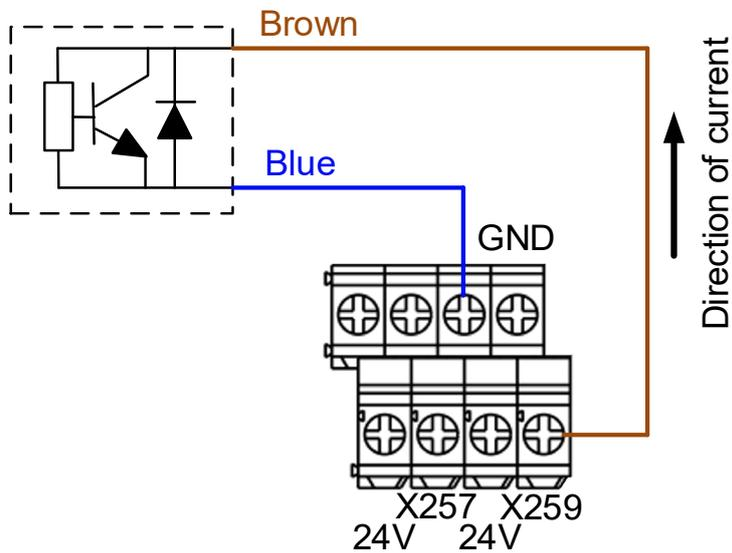
PNP 2-wire proximity sensor with polarity:
