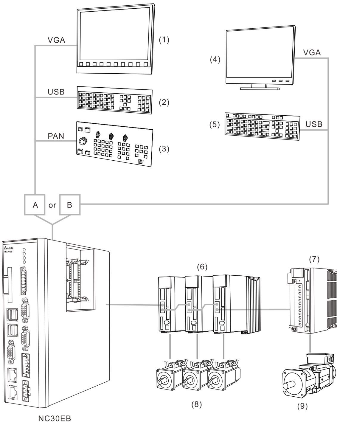
The NC series controller can connect to (6) ASDA series AC servo drives, (7) ASDA-S spindle servo drive, (8) ECMA series servo motors, and (9) ECMS series spindle servo motor.
