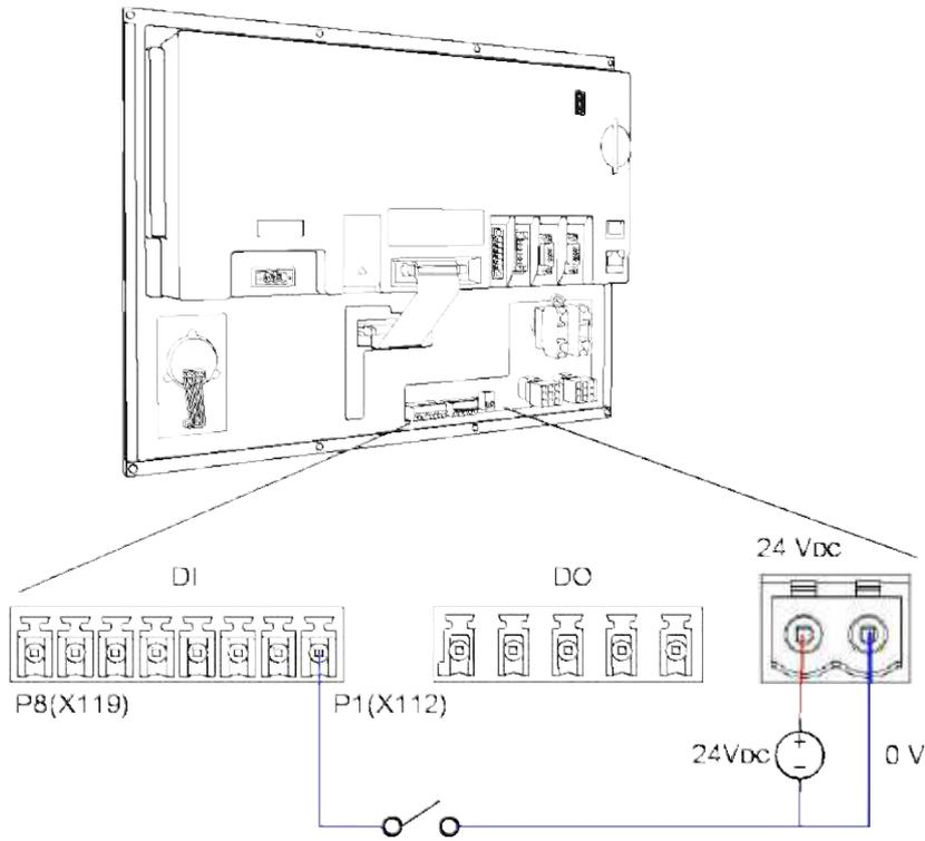
DO wiring (24V power is supplied from machine operation panel B)
