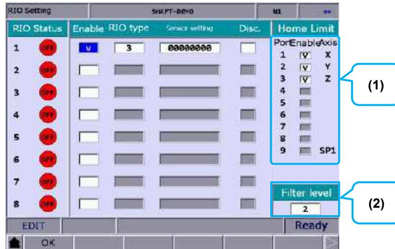
(1) Axis selection: positive limit DI, negative limit DI, and home DI of X - A axes are input from the AXIS 1~4 connector on the controller (this connector is only available on NC3XX series models). According to the selected axes, each axis takes three DI points from X256, which are positive limit DI, negative limit DI, and home limit DI respectively.
