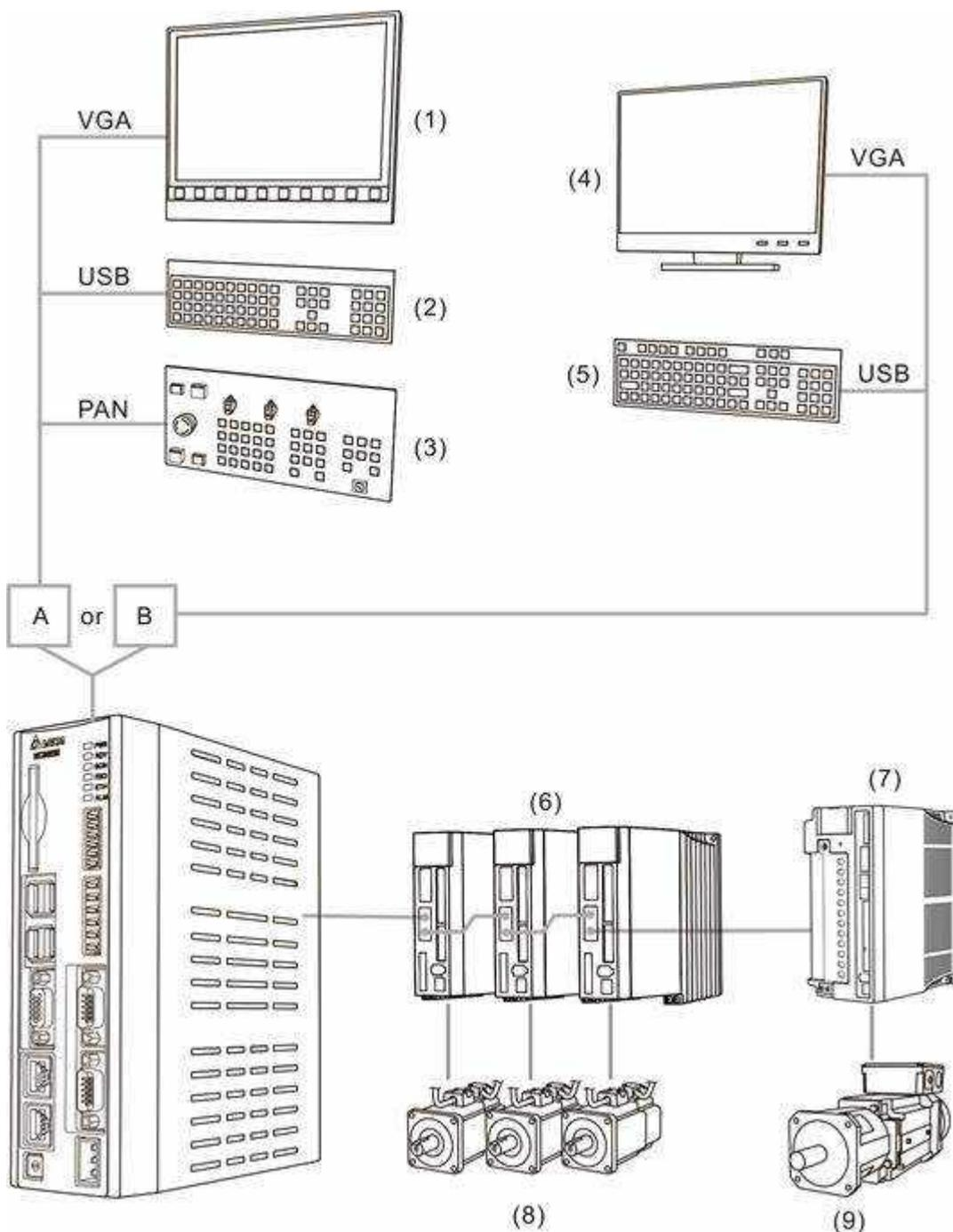
The NC series controller can connect to (6) ASDA series AC servo drives, (7) ASDA-S spindle servo drive, (8) ECMA series servo motors, and (9) ECMS series spindle servo motor.
